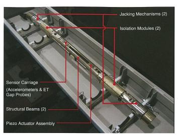
**Figure 5**. MODAR tool head with major subsystem identified
