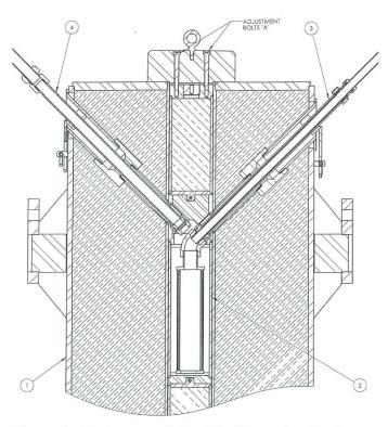
Figure 8. Canister and Flask in Operating Mode
