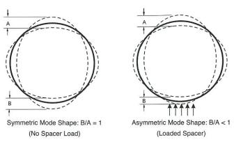
**Figure 2.** PT mode shape asymmetry resulting from a loaded spacer
