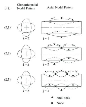
**Figure 4.** PT shell mode shapes and resulting spacer motion
