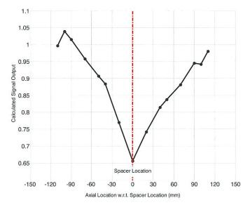
**Figure 3.** Typical MODAR system response to a loaded spacer
