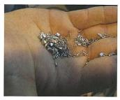
Figure 6. Chopped Detector Particles
