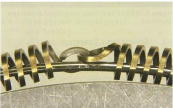
**Figure 1.** Optimized tight fitting annulus spacer installed on a pressure tube
